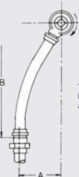
The correct way to install the hose on a rotary union
